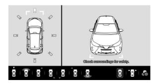
When the SMOD warning line appears, the button will temporarily disappear. Display button when SMOD warning line disappears. The SMOD warning appears during the rotation of the vehicle icon, the vehicle icon continue to rotate to the specified angle.
