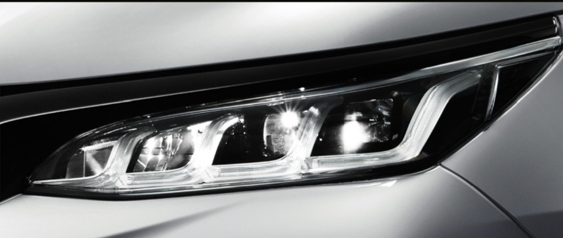
Quad LED Headlamps with LED Daytime Running Lights Greater sight and visibility for both night and day.
