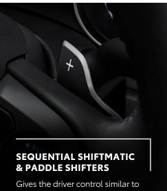
Gives the driver control similar to a manual car with excellent response, and allows the driver to shift the gears up or down while their hands remain comfortably on the steering wheel.
