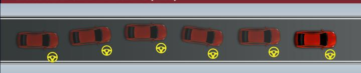
Constantly keeps the vehicle centred in its lane by actively applying slight corrective steering.
