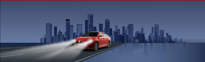
Detects headlights of oncoming vehicles and proximity of taillights and switches automatically between low and high beam.
