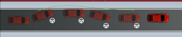
Automatically makes corrective steering to help driver keep the vehicle in its lane. Alerts the driver via the display and audio buzz.
