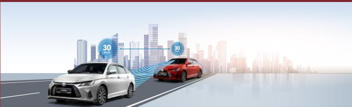
Detects speed and distance of vehicles in front to automatically adjust and maintain speed from a safe following distance.
