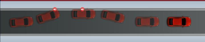
Detects when a vehicle is drifting out of its lane. Alerts the driver via the display and audio buzz.
