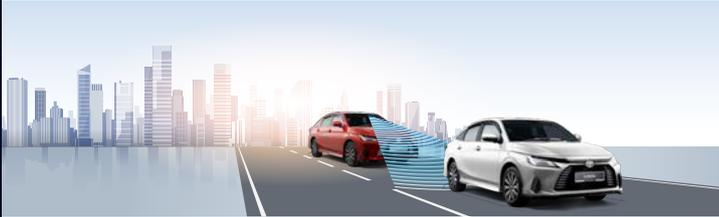
Uses Stereo Camera to detect potential collisions with other vehicles or pedestrians. Automatically apply the brakes to reduce the severity of a crash or prevent it.
